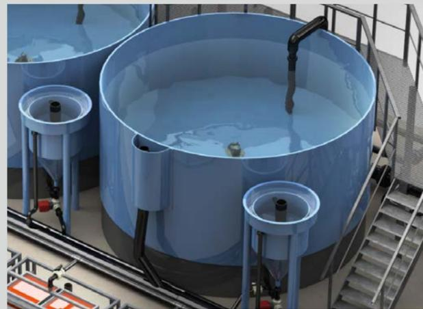
Particle separator and tank with double discharge through which 85 % of the water passes out through an auxiliary discharge and is brought to the discharge pipe. The remaining water is discharged through a centre discharge pipe in the bottom and must pass the particle separator before it is transported to the discharge pipe and cleaned in a mechanical strainer.
